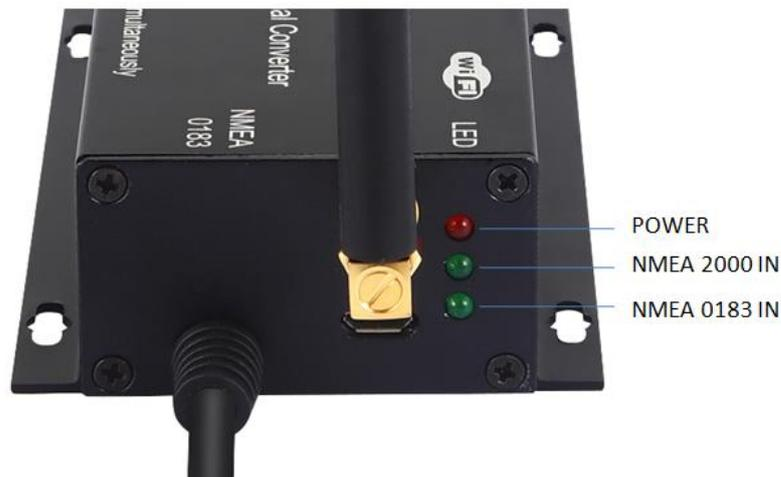
Figure 4: LED functions
