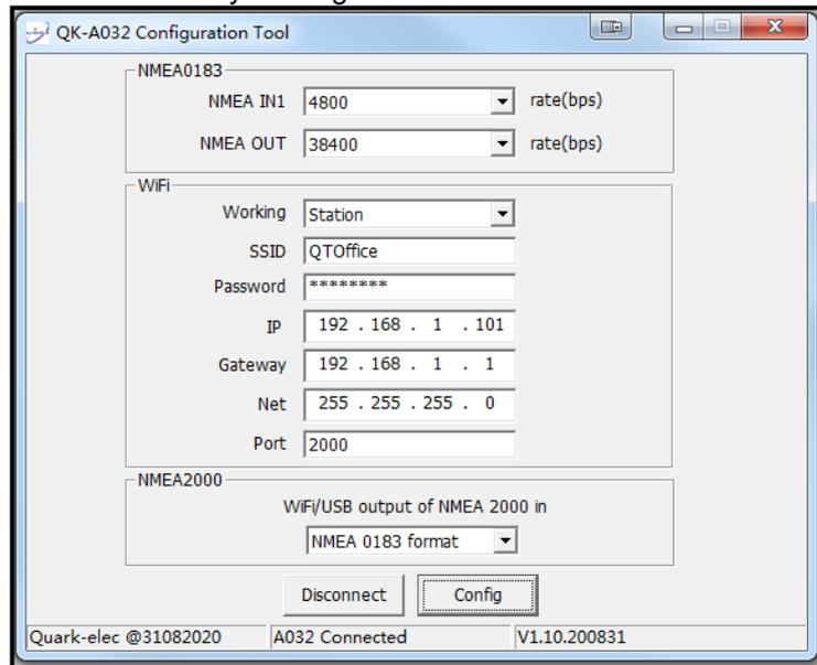
7. Enter the **router's IP address** in the **Gateway** section. This can usually be found on a label on the router. Leave the other settings as they are.
